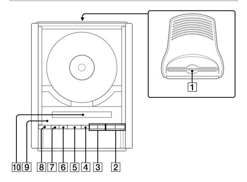
Display window 10 FUNCTION 7 (11, 17) OPEN/CLOSE ▲ 1 (11) Remote sensor 9 TUNER/BAND 6 (13) TUNING +/- 3 (13) VOL +/- 2
